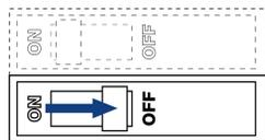
Verify that power has been removed to the light switch, by testing the switch, and by using a multimeter or other type of voltage tester before removing any wires from the switch.
